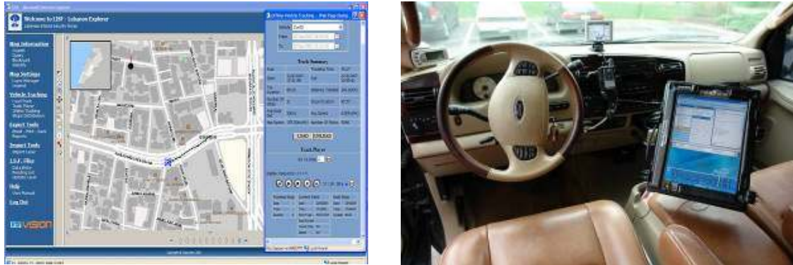
Figure 8: LISF GIS web-based tracking application allowing non-operations room personnel on the road to access GIS maps and track vehicles
